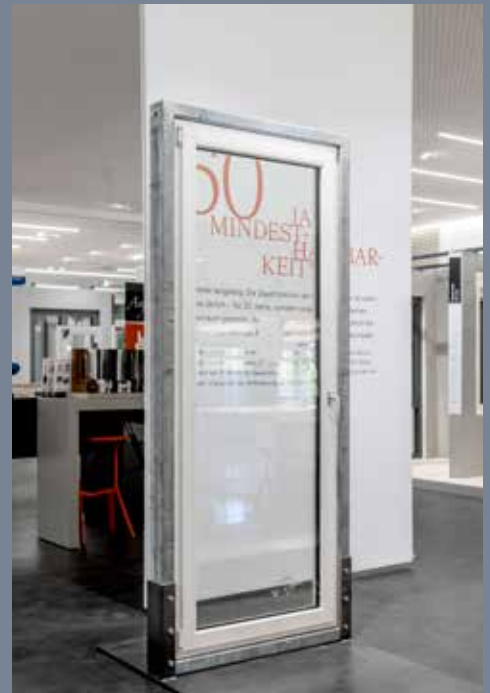
Repeated opening and closing test on a 90 x 230 cm Finstral aluminium-uPVC casement door, carried out at the Institut für Fenstertechnik (ift) Rosenheim with 65,000 cycles to the relevant test standard (EN 12400:2002-10); this is equivalent to over three times the RAL Quality Assurance Association requirement.
